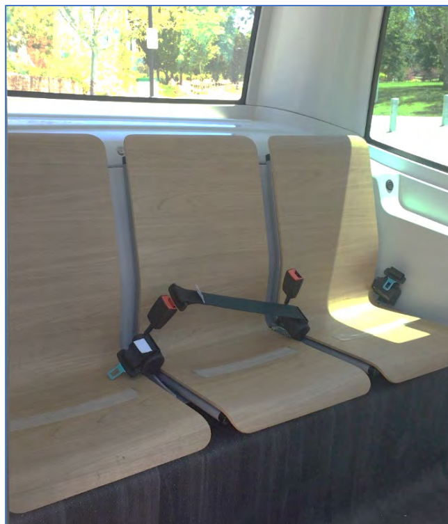
Figure 46: Seatbelts and Less Slippery Seating Surfaces Installed on the Shuttle
