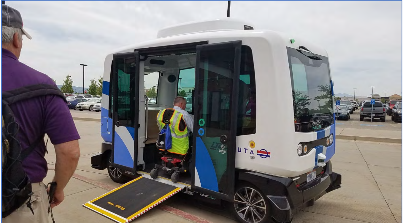
Figure 43: Ramp in the Deployed Position
