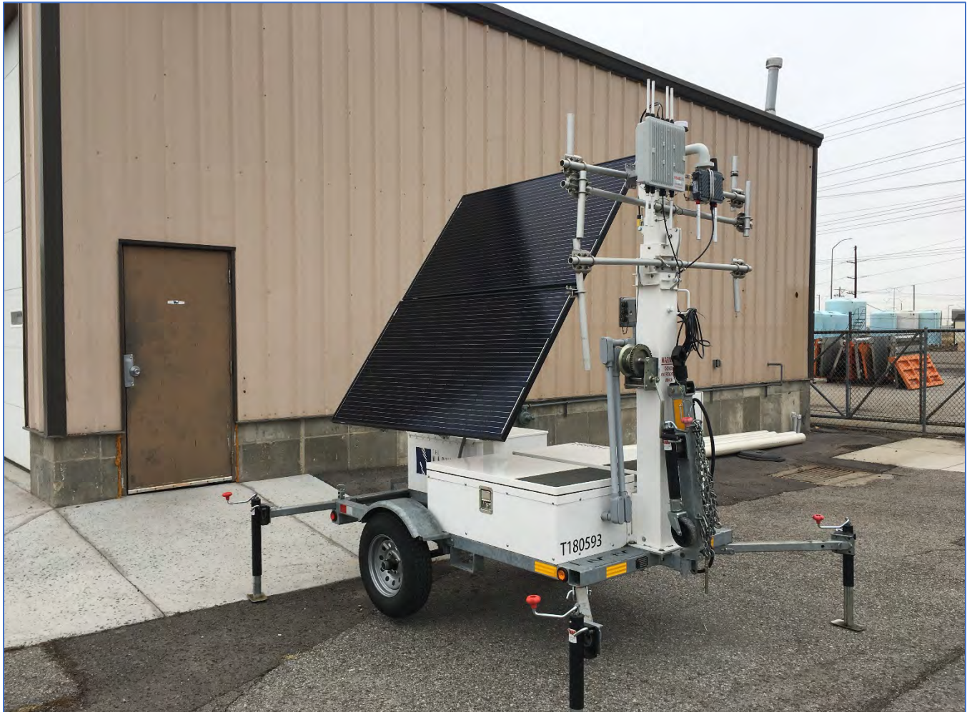
Figure 47: Portable Traffic Signal Controller and Roadside Unit
